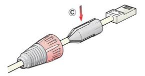
© Put the chuck onto the cable.
