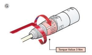
© Slide the boot to the housing and tighten the bushing (max. torque 3 Nm).
